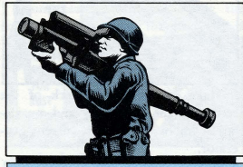
HOLD TRAINER LIKE THIS DURING SPINDOWN. PREVENTS DAMAGE TO GYRO.
