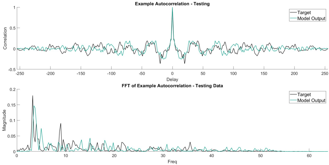
Fig. 28.: An example of the autocorrelation function of a less accurate model output (testing data) compared to the corresponding actual EEG for Participant 13. The Fourier Transform of both autocorrelation functions is shown below.
