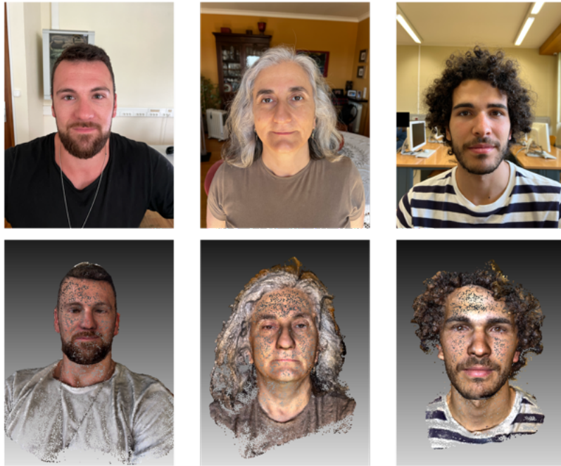
FIGURE 4.2: Illustration of three point cloud and image pairs for three subjects from the iPhonePLYv3 dataset.
