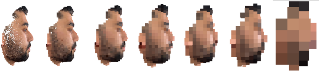
FIGURE 4.16: Voxel grid generation with voxel sizes ranging from 0.0025 to 0.150 with 0.0025 increments, spanning from 7812 voxels down to 49 voxels.
