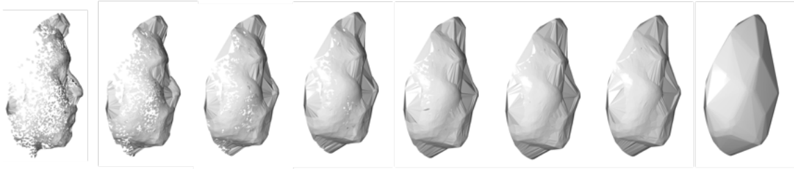
FIGURE 4.25: PMP initial point cloud to mesh conversion for subject id_001. From left to right, the parameter alpha starts with 0.02 with an increment of 0.01 until 0.07. The furthest image to the right is the convex hull.
