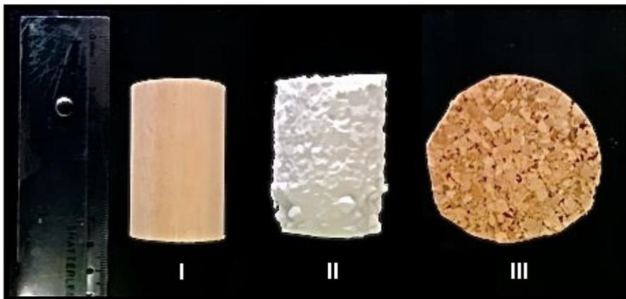
Fig. 1 – Selected substrates tested in this study: I – wood; II – styrofoam and III – cork.
