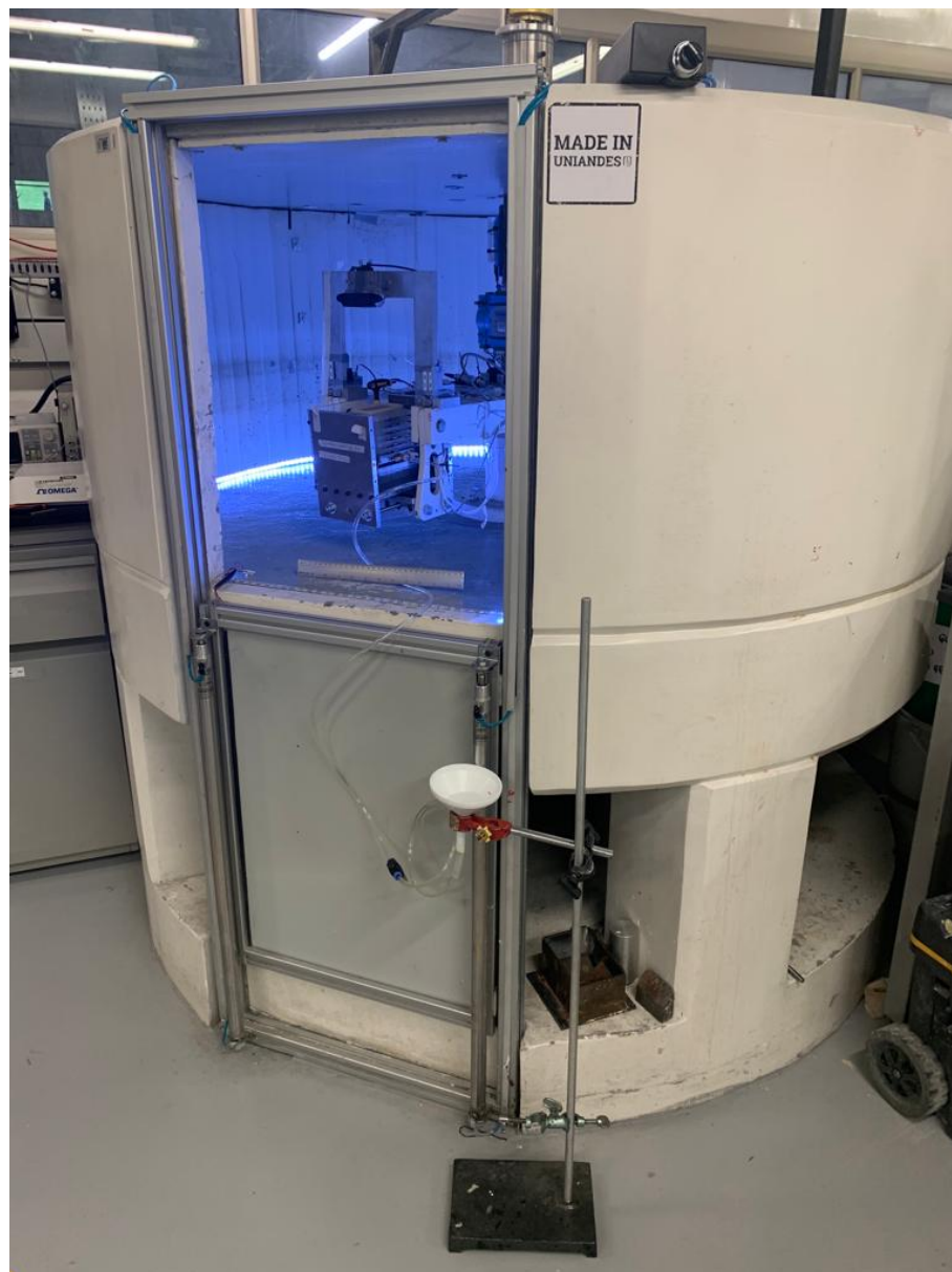
Figure 7.3: Illustration of the induced partial saturation process in the geotechnical centrifuge by soil desaturation
