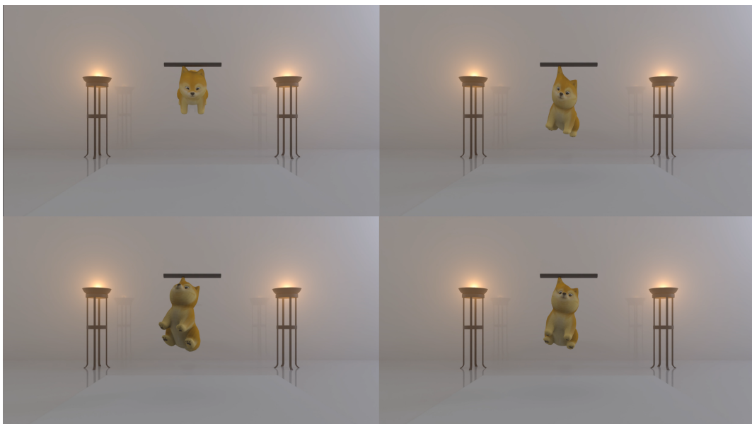
Figure 5.6: A volumetric model is hanged under constant gravity with multiple vertices fixed to a pole. The conditions are \alpha=0.000005 , iteration count = 50, damping coef. = 0.2 and step-size= \frac{1}{24}
