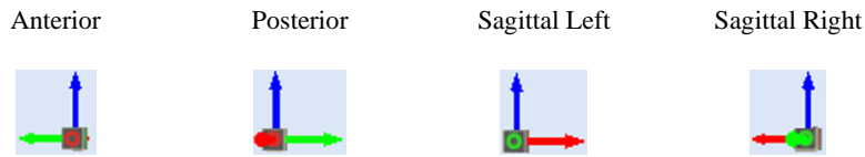
Figure 18 – The Xsens Coordinate System of the different view perspectives.
