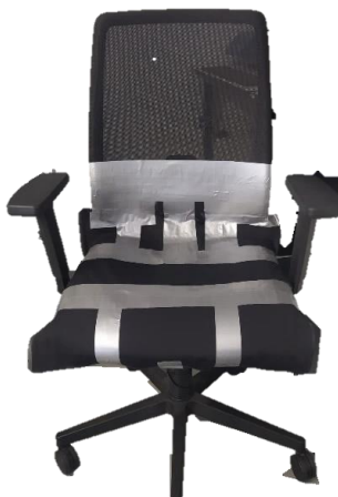
Figure 17 – Setup of the Pressure Mat on the office chair.
