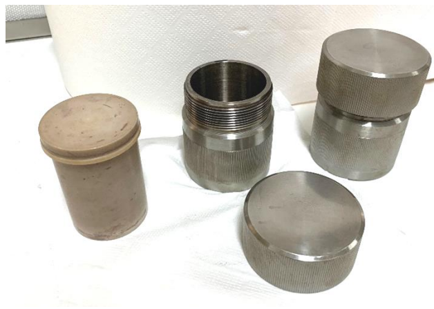
Figure 33 - Used autoclave system for the preparation of the coatings through the hydrothermal method.
