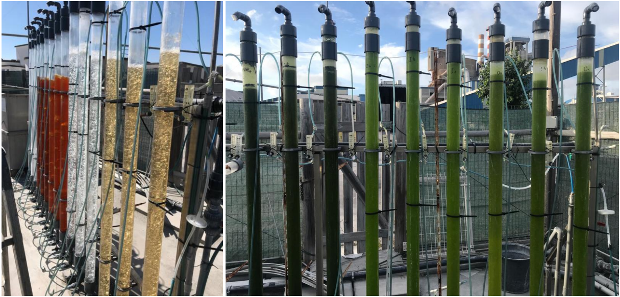
Figure 11: Bubble columns with each specific nutrient solution, prepared to receive the inoculum (right). Bubble columns' final appearance after receiving the inoculum (left).
