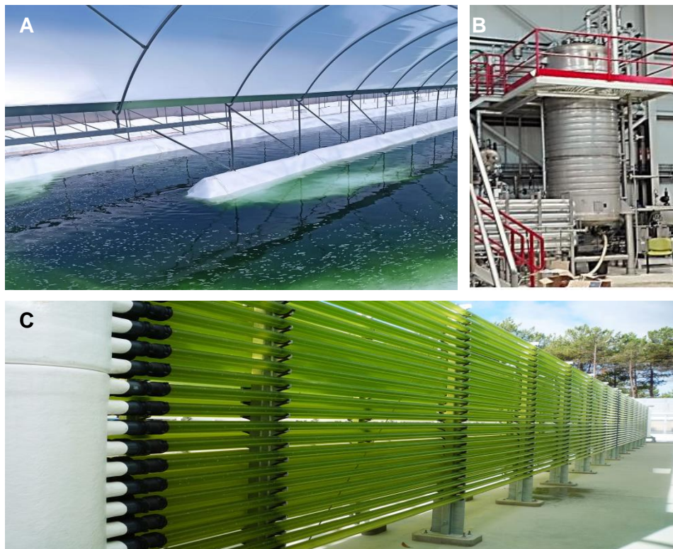
Figure 3: Different microalgae cultivation systems from Allmicroalgae (Pataias). (A) Open pond system 200 m 3 ; (B) Closed bioreactors 90 m 3 (PBR); (C) Industrial 5 m 3 Fermenter.
