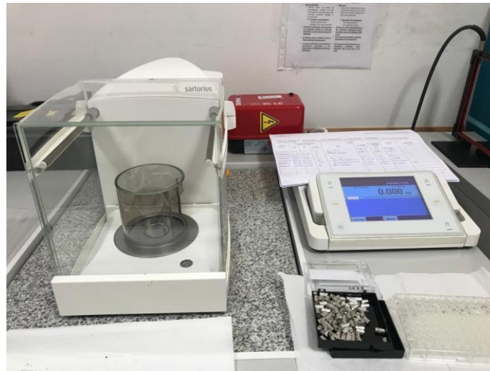
Figure 14: Sartorius precision balance used to weigh the aluminium capsules with the sample.
