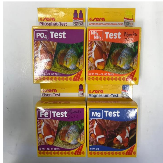
Figure 10: Aquarium Sera Kits used to quantify the concentration of phosphate, ammonia, iron and magnesium.
