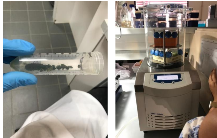
Figure 12: Samples after being freeze-dried (left) and a freeze-dryer, CHRIST Alpha 1-2 L Dplus (right).
