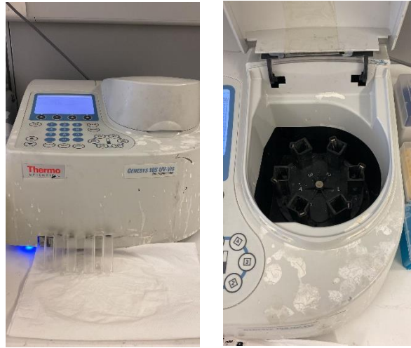
Figure 6: UV/vis Genesis 10S spectrophotometer with quartz cuvettes in front of it (left) and its interior (right).
