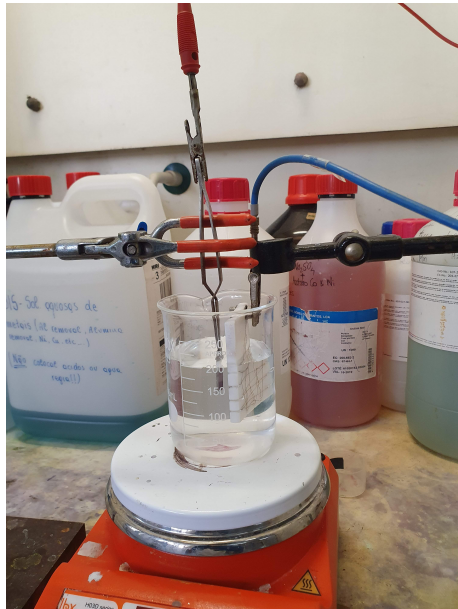
FIGURE 2.1: Photograph of the electropolishing setup used.
