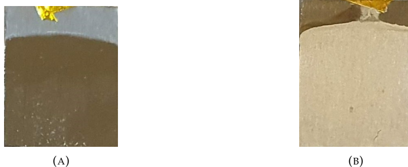
FIGURE 3.3: W EP results obtained using 10V, 30 minutes and 0 rpm for a) 0.125M NaOH electrolyte and b) 0.5M NaOH electrolyte.
