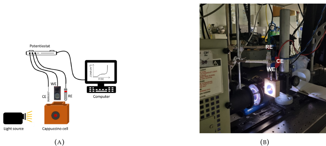
FIGURE 2.6: a) Schematic representation of j-V measurement system [94]. Photographs of measurement with a solar simulator under b) 1-sun light [40].
