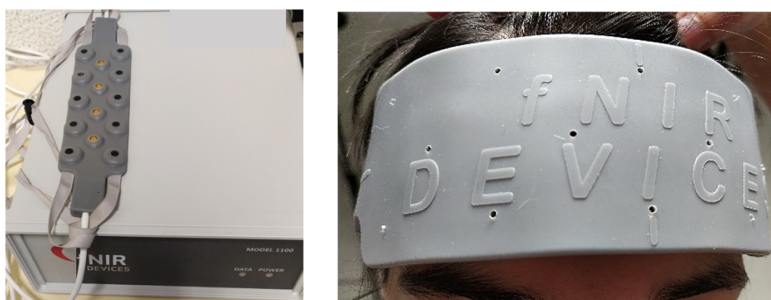
Figure 6.1. fNIR100A-2 device attachment in the participant head – prefrontal cortex region.
