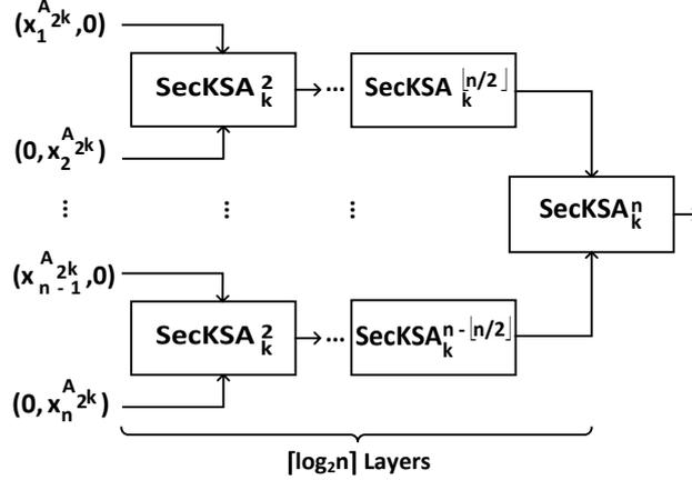
Figure 1: High-order A2B conversion based on Carry-Propagation adder.
