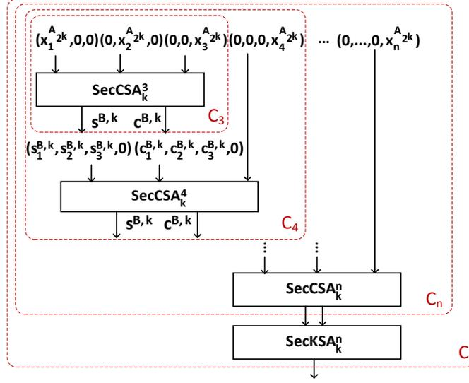
Figure 5: High-order A2B conversion based on Carry-Save adder.
