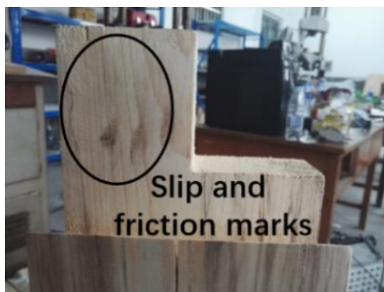
Fig. 12. Slip and friction marks
