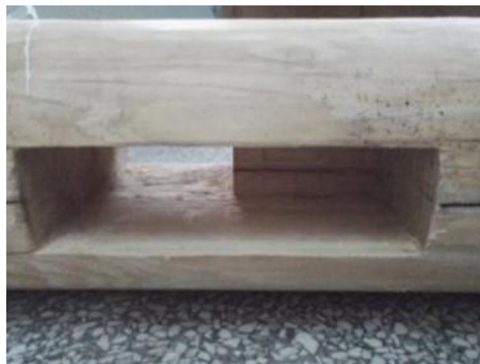
Fig. 18. The mortise after loading is completed
