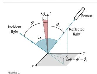
Viewing geometry convention:  $\theta_{v}$  and  $\phi_{v}$  are the zenith angle and azimuth of the viewing direction,  $\theta'$  and  $\phi'$  are the zenith angle and azimuth of a given illumination direction.  $\theta_{N}$  is defined as the zenith angle of the vector normal to a given wave facet, and  $\alpha$  is the phase angle between the incident and viewing directions.
