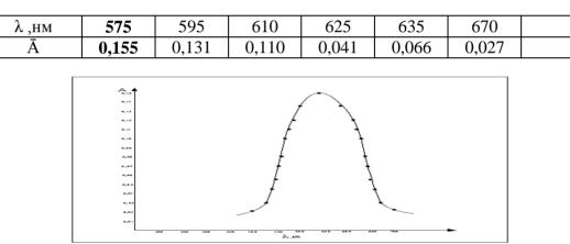
Dependence of the optical density of the complex of cobalt Yun 4- sulfo- $\beta$ -nitroso- $\alpha$  -naphthol on the tyolkin length
