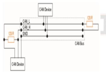
Fig.2 Implementation of CAN bus
