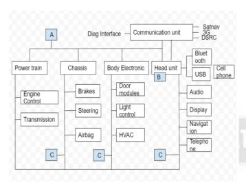
Fig 7. Possible locations for IDS deployment in the CAN bus system. A) CAN, B) ECU, C) gateways.
