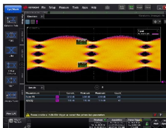
Figure 7. The Eye Pattern of 200G PAM4 EML in 800G Optical Transceiver. Clear Eye Opening and Good TDECQ are Demonstrated
