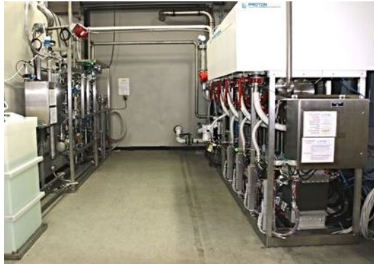
Figure 4: Cost breakdown of stack and photo of Proton MW electrolyzer
