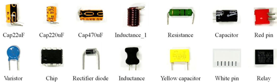
Figure 7. categories of electronic components and corresponding pictures.
