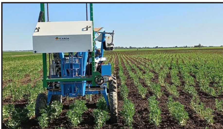
Figure 3. Phenomobile system working in faba bean field.
