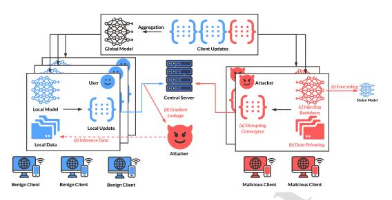
Figure 1: An Overview of Common Vulnerabilities in FL. Malicious attackers can: (a) manipulate model updates to prevent the global model from converging; (b) tamper data labels to induce erroneous predictions after training; (c) inject backdoors into the global model; (d) reconstruct data or inference data properties by eavesdropping model updates; (e) steal the global model while contribute nothing.
