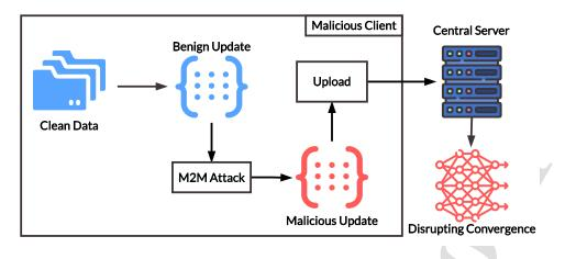
Figure 4: An illustration of M2M attack.
