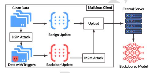
Figure 11: A High-level View of Injecting Backdoors with a Composite Attack. The attacker chooses a preferable trigger and tampers local data with the trigger. Local model is also trained on clean data to avoid detection. Most attacks aim at poisoning the global model with only a few clients.
