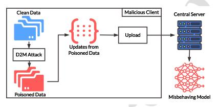
Figure 2: An illustration for D2M attack.
