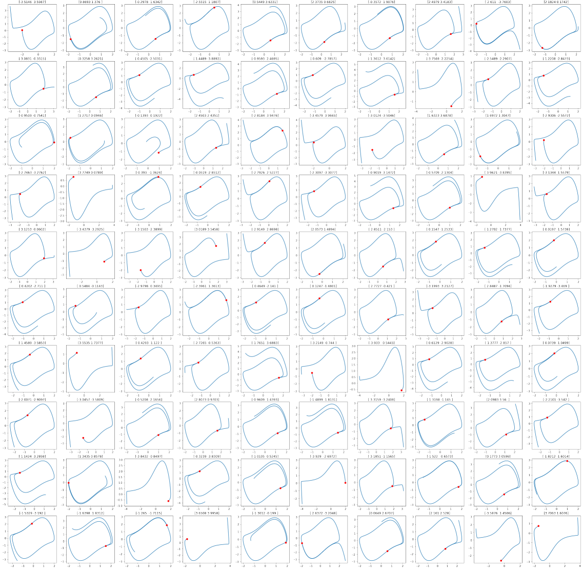
Figure 3.23: 100 Instances of the Van der Pol oscillator. The Van der Pol oscillator was generated using a random uniform distribution containing 100 values between [-4, 4] for the state variables x_1(t) and x_2(t) .
