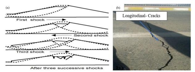
Fig. 11 - (a) The behaviours of the embankment dam during earthquakes, and; (b) cracks on the road of Darbandikhan Dam crest after the earthquake of November 12, 2017 [38]
