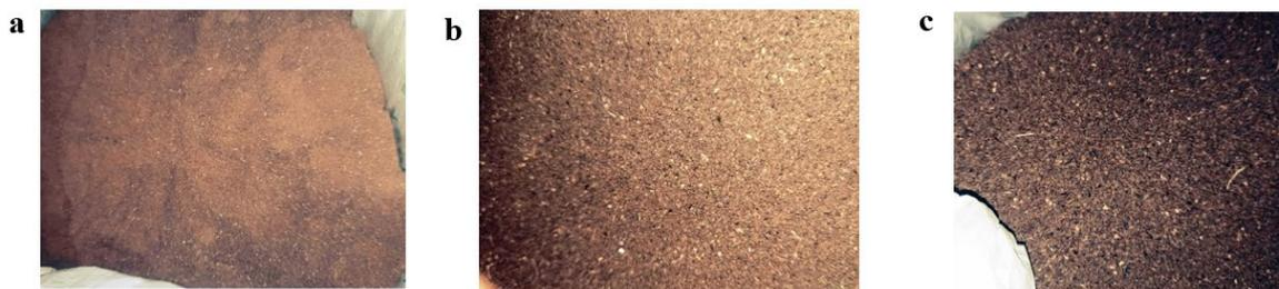
**Fig. 1 - Palm Kernel in Different Particle Sizes (a)  $< 0.6$  mm; (b)  $0.6 \leq x \leq 0.8$  mm; (c)  $0.8 < x \leq 1$  mm**
