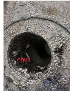
Fig. 3 - Coke formed on the wall of the reactor
