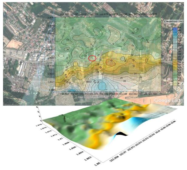
Fig. 2 - Topography of SMK Munshi sub-catchment area with its 3D surface elevation
