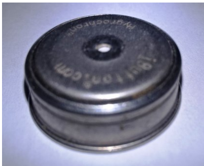
Figure 2 iButton for monitoring air temperature and relative humidity.
