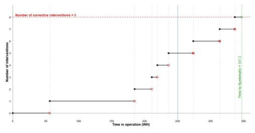
Figure 10. Counting processes applied to TAG 5513 truck for first systematic intervention.
