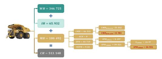
Figure 11. TAG 5513 truck hours categories breakdown.
