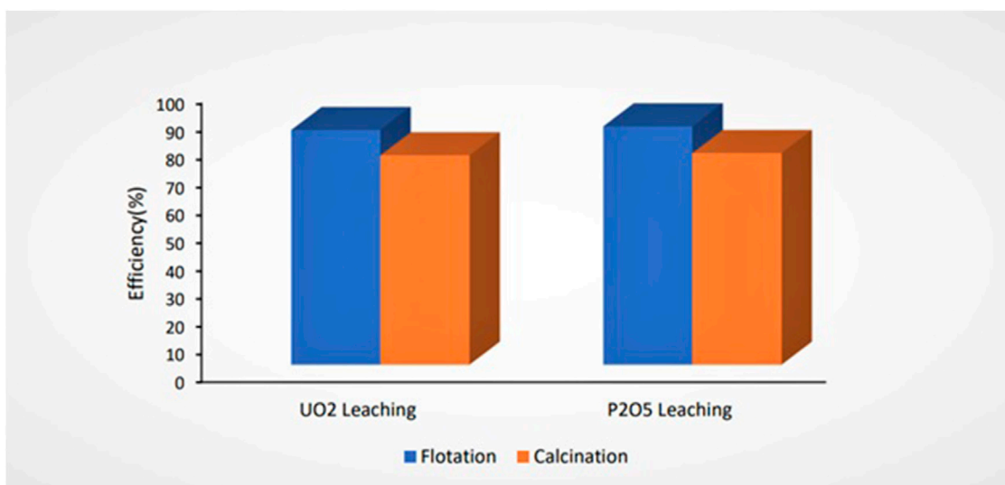
FIGURE 9 Effect of pre-treatment methods on uranium leaching efficiency (L/S = 5, time = 4 h, sulfuric acid concentration = 3 M, and T = 80°C).
