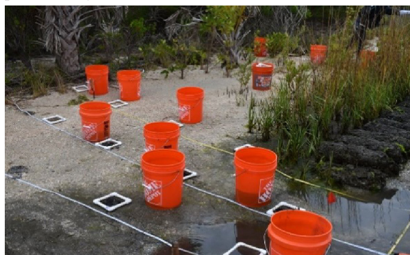
Figure 2. Sediment collection setup including quadrats and buckets placed along vertical transect lines.
