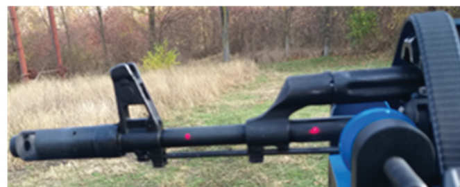
Figure 2. LT CT laser spots on barrel surface.
