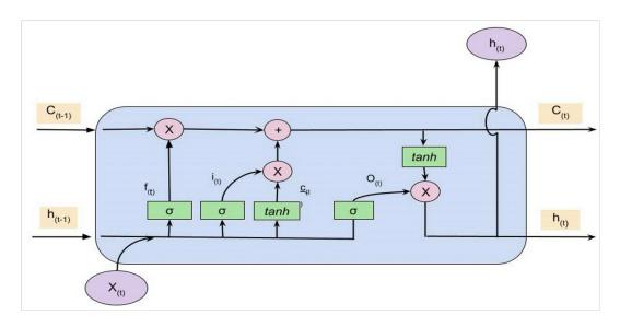
**Figure 2:** A LSTM model cell [21]; representing the workflow inside one particular cell. Input data  $x_{(t)}$  are fed into the cell which undergoes several activation gates  $\sigma$  and hyperbolic tangent function (tan h) and thus generates forgate gate  $f_{(t)}$ , input gate  $i_{(t)}$ , update cell  $c_{(t)}$  and output gate  $O_{(t)}$  for the purpose of estimating the candidate memory gate  $C_{(t)}$ , hidden layer  $h_{(t)}$  which in turn fed into the next cell unit.
