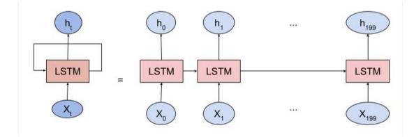
**Figure 3:** A simple representation of one of the LSTM layers used for building the learning model comprising 200 neurons. Every neuron of the layer is fed with unit of input data  $X_{(t)}$  to predict the hidden output  $h_{(t)}$  which is also fed into the next neuron to predict  $h_{(t+1)}$  along with  $X_{(t+1)}$ .
