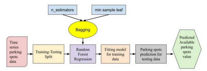
**Figure 4:** Workflow of Random Forest model. The time series data of parking spots availability has been split between training and testing data and used the training data to fit. The random forest regression uses the ensemble bagging method where the n\_estimators (=250) and minimum sample leaf value (=40) used as parameters here. Definite number of decision trees gets to be integrated for final predictions.
