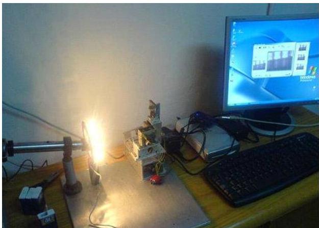
Fig. 4. Capturing images of screws with vision system
