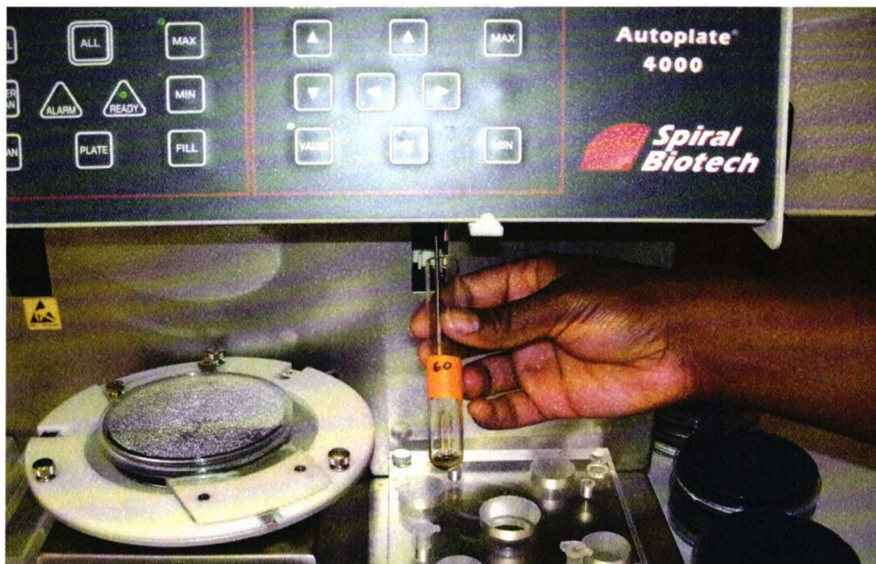
Figure 19. Spiral plater stylus obtaining sample from test tube
