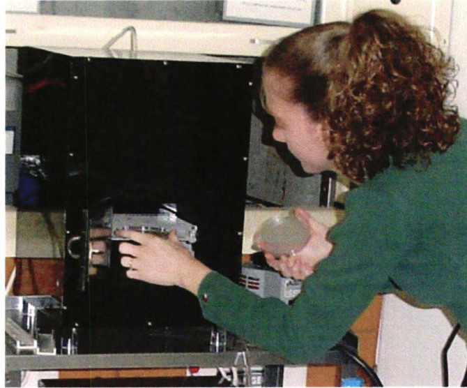
Figure 1. Placing Petri Dishes into Indirect Cold Plasma Chamber
