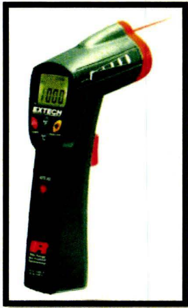
Figure 3. Extech Thermometer for External Temperature Measurement
