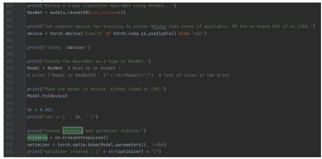
4. After that, device configuration is set. In this case, the virtual environment was configured using cuda interpreter.
