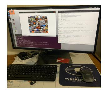
Figure 8: Jetson Nano configured and running the Fire-Smoke Classifier CNN.
