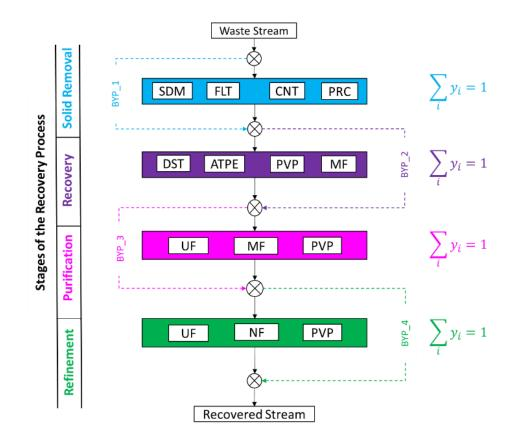
*Figure 21.* Superstructure for waste solvent recovery showing technologies, streams, and bypasses (SDM – Sedimentation; FLT – Filtration; PRC – Precipitation; CNF – Centrifugation; DST – Distillation; ATPE – Aqueous Two-Phase Extraction; PVP – Pervaporation; MF – Microfiltration; UF – Ultrafiltration; NF – Nanofiltration; BYP\_1,2,3,4 – Bypasses 1,2,3, and 4
