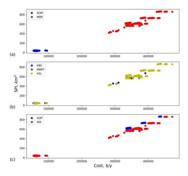
*Figure 20.* Distribution of technology selection for each stage. Subplots (a), (b), and (c) are for primary, secondary, and tertiary stages, respectively
