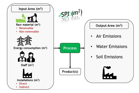
Figure 5. The various aspects to quantifying the sustainable process index
