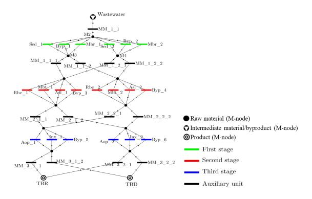
*Figure 18.* Maximal structure for coffee case study. TBR – To Be Recycles; TBD – To Be Discharged.
