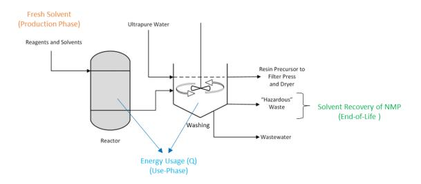
Figure 42. Flowchart for case study showing the different stages of NMP life cycle
