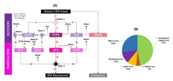
Figure 2: (A) A superstructure of the possible solvent recovery methods to separate IPA from the water. ATPE, UF, SDM, PVP, DST, and INCN represent aqueous two-phase extraction, ultrafiltration, sedimentation, pervaporation, distillation, and incineration, respectively. The most economically viable pathway for IPA recovery is highlighted in red. (B) The cost distribution of the optimal pathway (PVP1—UF2).
