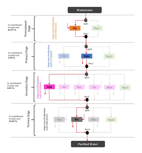
Figure 11. Optimal pathway for municipal wastewater treatment.
