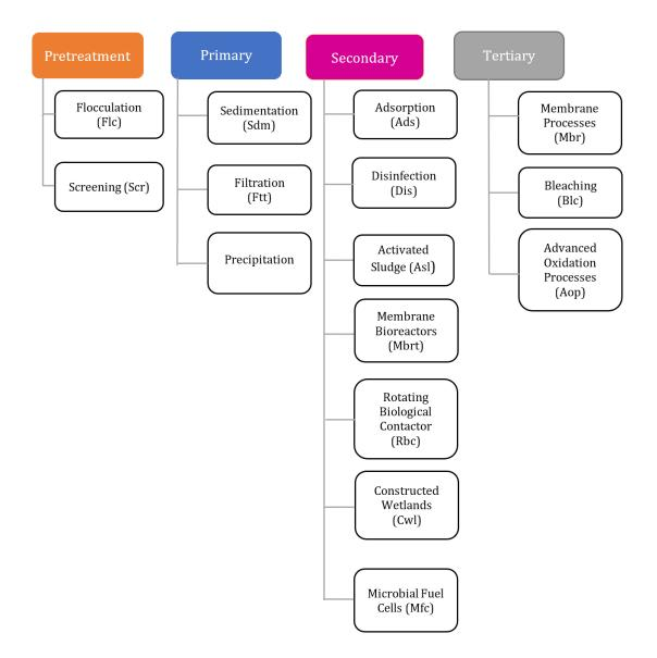
Figure 8. Typical technologies found in stage-wise WWT
