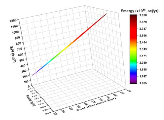
*Figure 26.* Sensitivity analysis showing how cost, SPI, and Emergy change with varying waste flowrate
