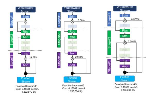
*Figure 17.* First three feasible structures showing selected technologies, the cost of treatment for 1 L of wastewater treated, and annual cost
