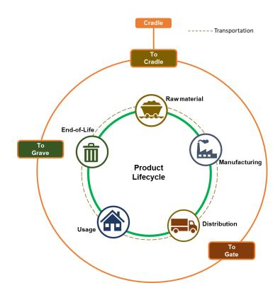
*Figure 2*. The product life cycle comprises various stages, each of which involves material transportation. LCA can be conducted using one of three primary models: cradle-to-gate, cradle-to-grave, and cradle-to-cradle
