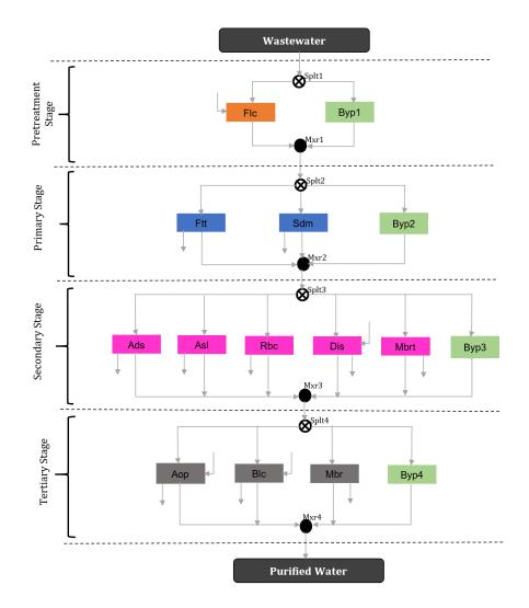
Figure 10. Generic superstructure for municipal and pharmaceutical wastewater treatment
