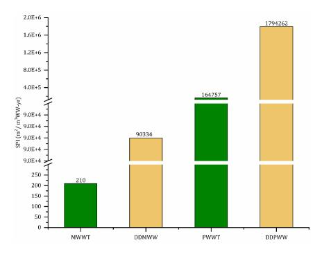
*Figure 13.* Consequential SPI for the various scenarios (MWWT – municipal wastewater treatment; DDMWW – direct disposal of municipal wastewater; PWWT – pharmaceutical wastewater treatment; DDPWW – direct disposal of pharmaceutical wastewater)
