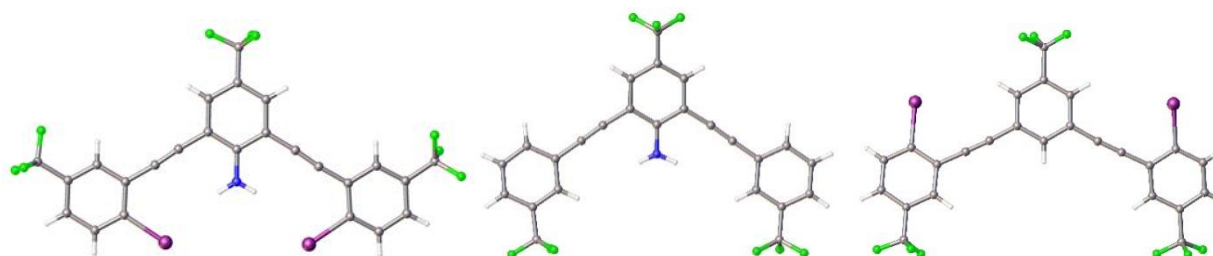
Figure 21. Crystal structures of G3XB molecule (left), G3HB (middle)*, and nHBeXB (right) highlighting the importance of the intramolecular HB to produce the bidentate conformation. *Representative example from the orthorhombic polymorph.
