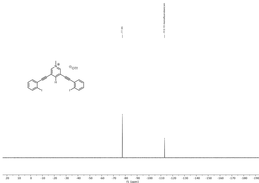
Figure S180. ^{19}\text{F} NMR spectrum of 3 (470 MHz, \text{CD}_3\text{CN} ). \text{C}_6\text{H}_5\text{F} (monofluorobenzene) internal reference.
