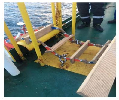
Additionally, a study was found to have been conducted by the University of Southampton to investigate the effectiveness and impact of various methods used to secure the ladders at intermediate lengths. It reveals that the use of shackles in pilot transfer arrangements had led to a series of damages. Finally, it concludes that the
