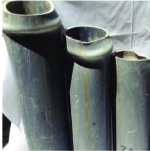
Figure 2-1 Failure of hollow tube due to Local buckling (Adbulla, 2021).
