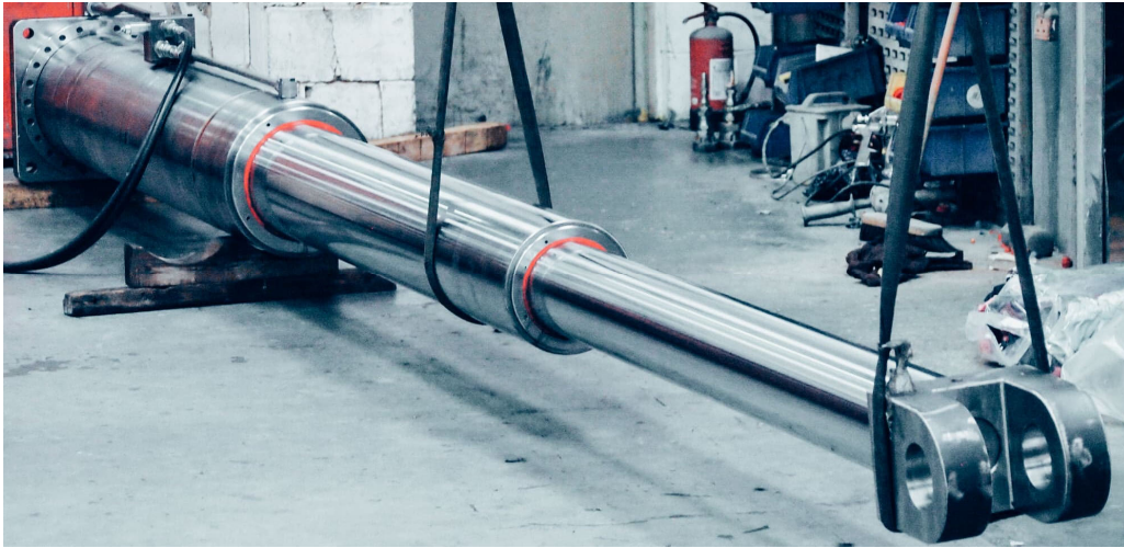
Figure 2-6 Telescopic hydraulic cylinder (Apex Hydraulics, 2016)
