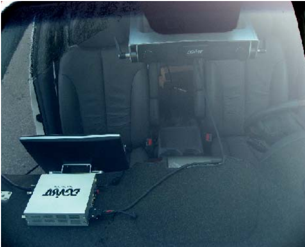
Figure 5. Stereo vision system mounted on vehicle
