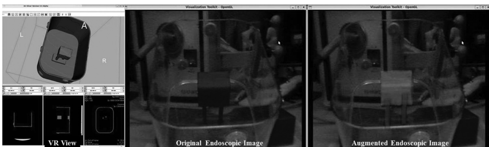
Figure 7. The left image is a 3-D rendering view (VR view) and the middle is the original endoscopic image. The right image shows the resulting overlaid 3-D surface model data on the endoscopic image. Evaluation was conducted using the raw endoscopic images and the augmented endoscopic images.
