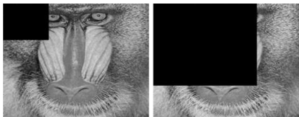
FIGURE 13. Occluded watermarked images. Left: watermarked image with 10% area occluded. Right: watermarked image with 50% area occluded.
