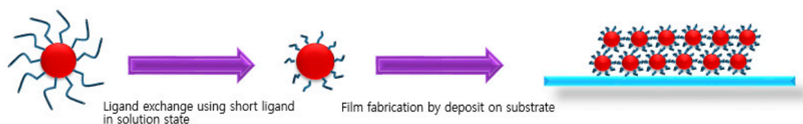
Figure 5. Schematic of the solution-phase ligand exchange and film fabrication. Ligands of CQDs are exchanged in the solution-phase first. After that, CQD films can be fabricated just by spin-coating the CQD inks on the substrate.
