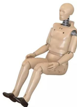
Figure 1-3 FAA Hybrid III 50th percentile male dummy (ATD) (Adapted from Wikimedia commons)[18]
