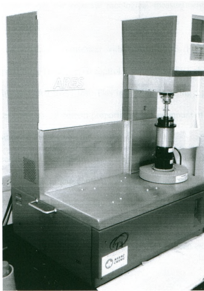
Figure 3.10 ARES rheometer used for rheology measurements.
