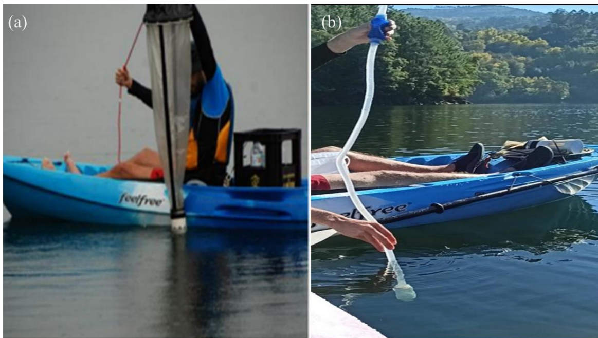
Figure 2.2 - (a) Zooplankton sampling with a plankton net of 153 \mu\text{m} ; (b) Pumping system for phytoplankton sampling.
