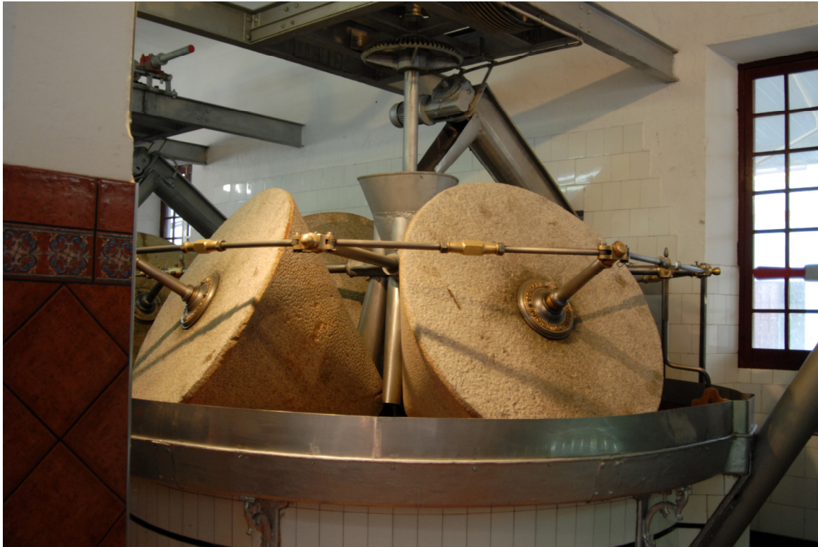
Figure 1. Conical stones olive oil mill.
