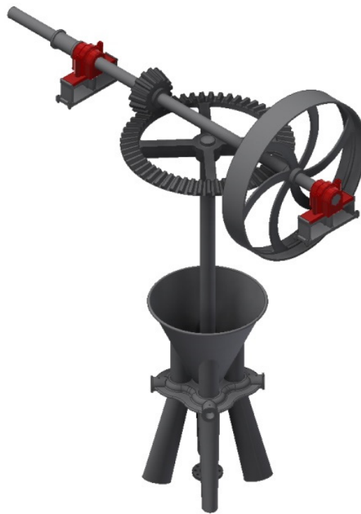
Figure 4. Motion transmission system in the conical stones olive oil mill.
