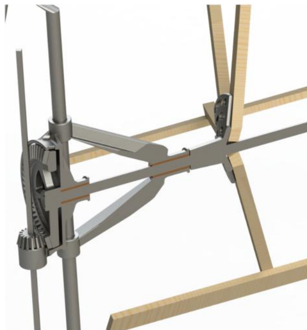
Figure 8. Sectional view of the sheaf pusher system.
