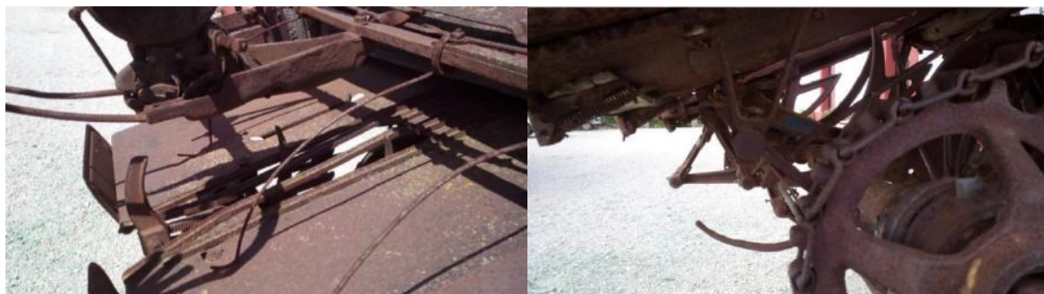
Figure 21. System of knotting and compacting needles: top view (left) and bottom view (right).
