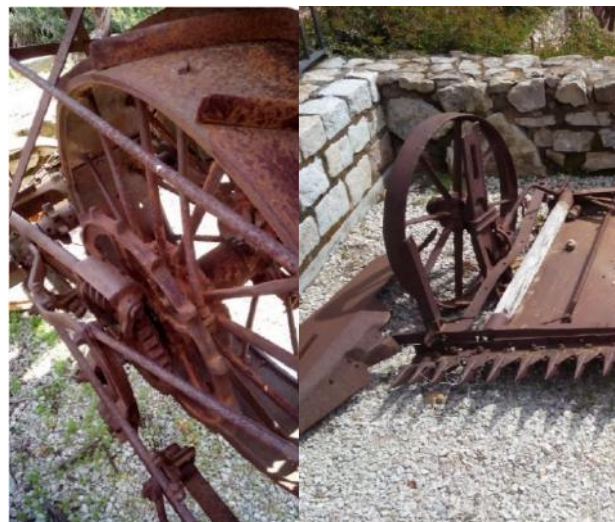
Figure 29. Drive wheel (left) and drag wheel (right) with adjusting levers.
