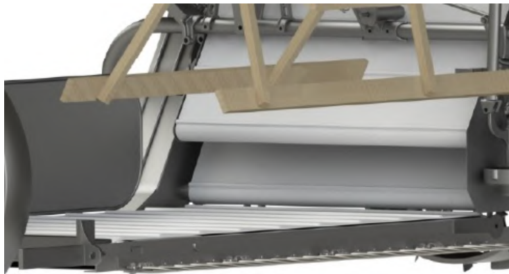
Figure 11. Bottom view of the rise conveyor system of the sheaves.
