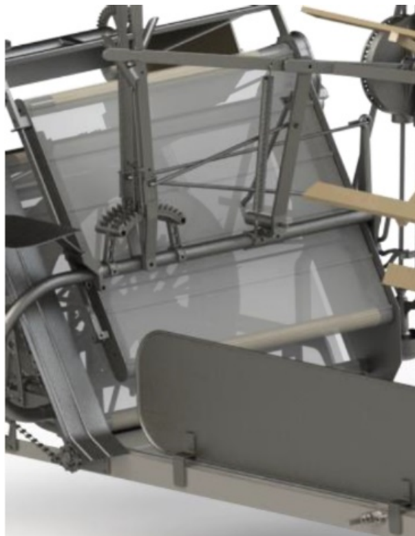
Figure 10. Top view of the rise conveyor system of the sheaves.
