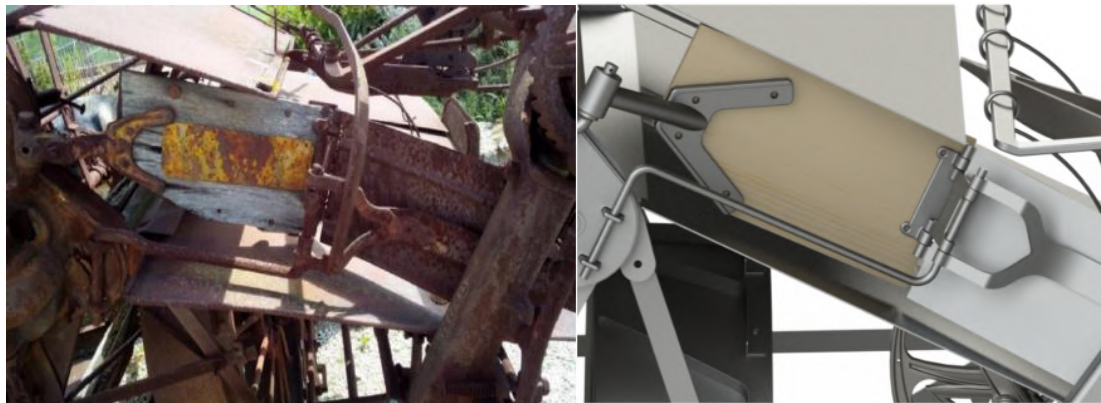
Figure 19. Sheaf grouping system (left) and 3D CAD model (right).
