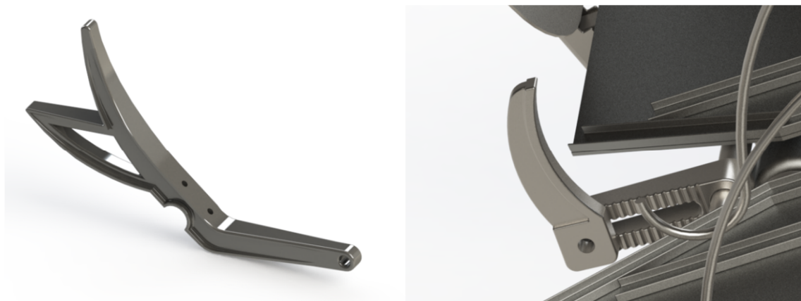
Figure 22. Compacting needle ( left ) and trigger of the knotting system ( right ).
