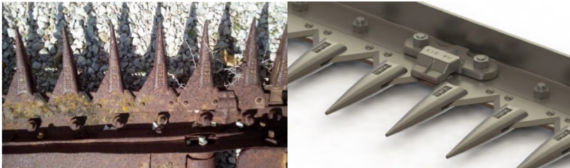
Figure 4. Cutting system with tines and blades (left) and its computer-aided design (CAD) three-dimensional (3D) model (right).
