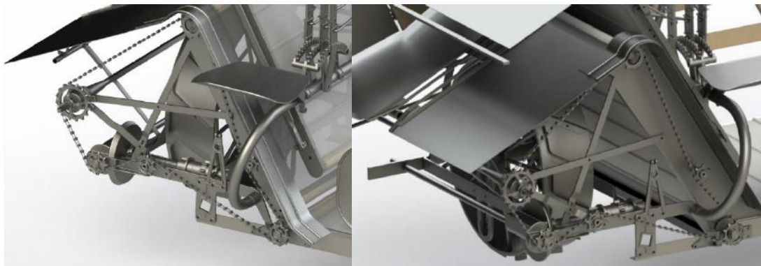
Figure 25. Mechanical transmissions: back view (left) and front view (right).
