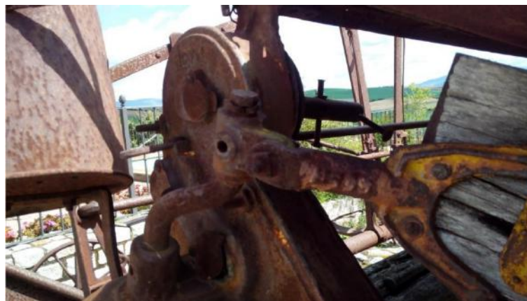
Figure 20. Connecting rod/crank mechanism in the sheaf system.
