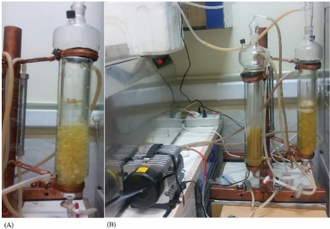
Figure 5. (A) Culture of G. lucidum in bubble column bioreactor, (B) co-culture of G. lucidum and B. subtilis in bubble column bioreactor.
